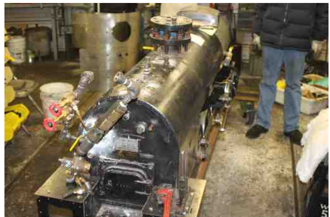
534 showing some of the piping on the backhead
