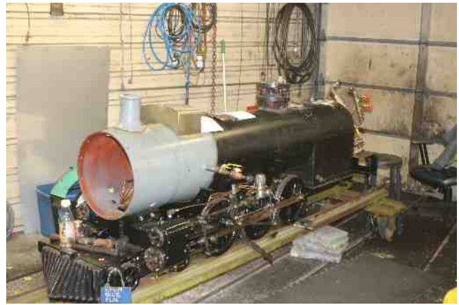
534 with the new boiler and firebox mounted
